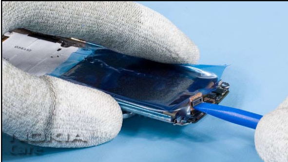
25. Open the flex connector of the LCD.
